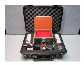
The **Paladin EZ Logger** is a compact, single-channel, wireless transmitter that provides continuous, real-time, In-mold Temperature Measurement throughout the heating and cooling cycles. Its compact design is simple to mount on molds or spiders and easy to operate. This affordable, data logging device will satisfy your need to know what is happening inside the mold *as it happens*.
