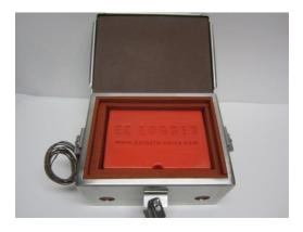
**System Components** - Stainless steel insulated box, four rotomolded Ambient-Temperature Heat-Sinks, 3 Type-K thermocouple sensors, wireless transmitter with antenna & spare battery, receiver device with high-gain antenna, I/O cable, hand tools, and carrying/storage case to provide protection from water, dust, sand and impact.
